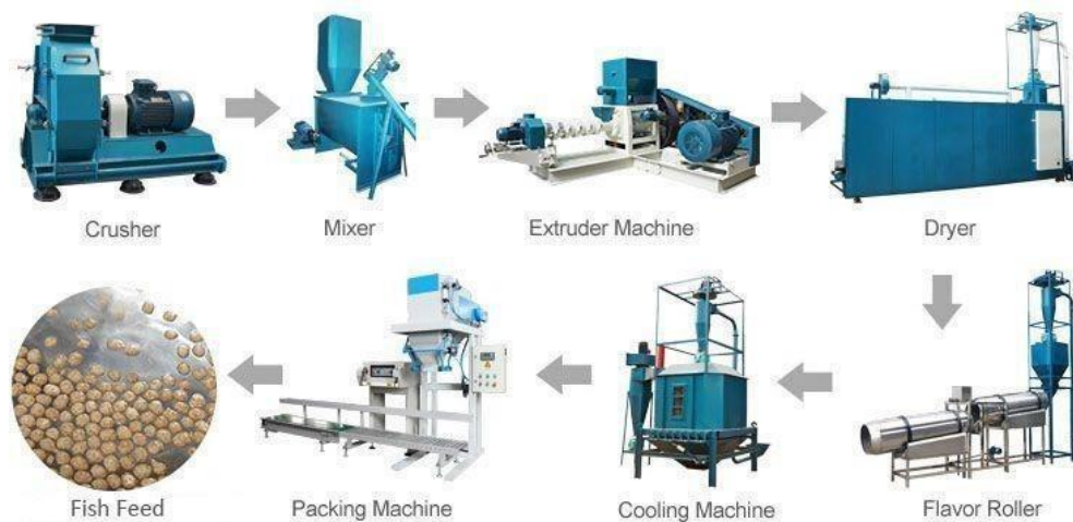
FIGURE 9: MODEL ILLUSTRATION OF A FISH FEED MILL
